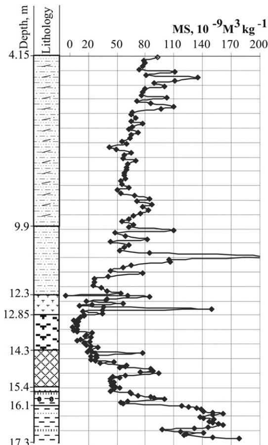
Fig. 7. Distribution of magnetic susceptibility in Netiesos section (magnetic susceptibility,  $\times 10^{-9} \text{ m}^3 \text{ kg}^{-1}$ /depth of samples, m). For lithological description, see Fig. 8.
