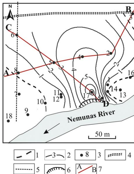
**Fig. 3.** Distribution of the Merkinė (Eemian) interglacial sediments in the Netiesos environs. 1 – limit of the Merkinė interglacial sediments distribution; 2 – isoline of sediment thickness (m); 3 – borehole and its number; 4 – road; 5 – clearing; 6 – outcrop; 7 – cross-section.
