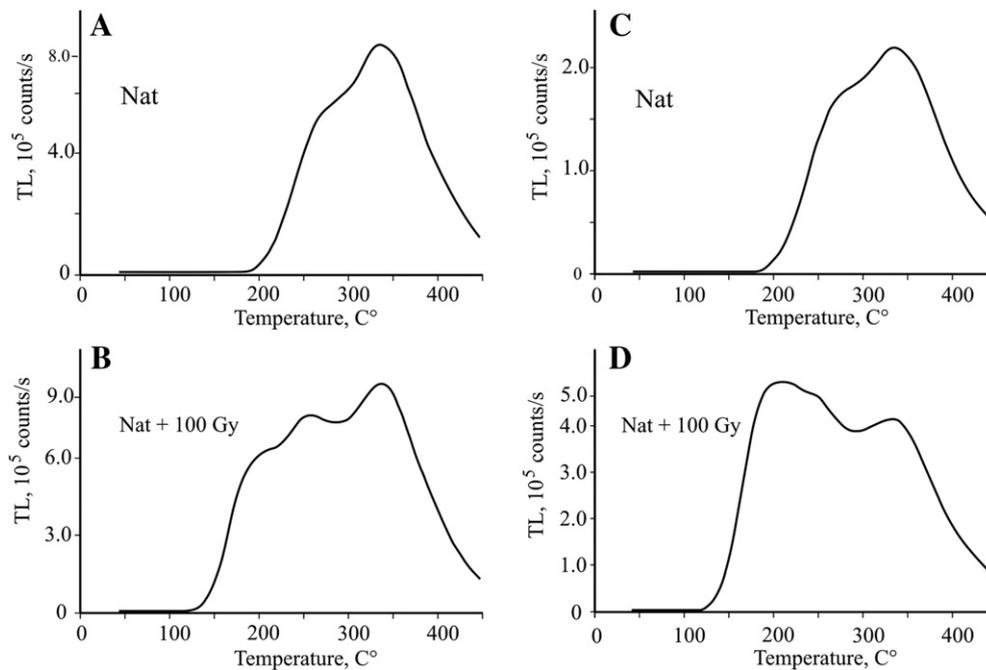
**Fig. 9.** Typical TL glow curve shapes for natural (A) and irradiated to 100 Gy (B) potassium feldspar extracted from the sediment samples N-4–N-10 taken from the depths between 12.9 and 4.6 m (91.1–64.4 ka). TL glow curve shape for natural (C) and irradiated feldspar (D) from the sediment sample N-11 taken at a depth of 3.9 m (20.4 ka) is considerably different.
